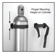
Hold Cylinder Safety Wall Bracket against the wall in the desired location, and outline mounting holes with a pencil. The bracket should be mounted so that the Velcro® strap is just below the crown of the cylinder.
