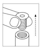
**STEP 1.** Remove the bolts from the base of the safety stand Upright Support.
