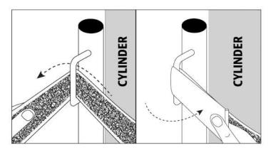
**Step 4.** Roll the cylinder into the safety stand until it is touching the upright supports. Orient cylinder valve outlet so it is facing to the left. Place bottom Velcro® Safety Belt around cylinder and through loop. Tighten belt securely. Repeat with top belt. Cylinder should be very tightly attached to stand.
