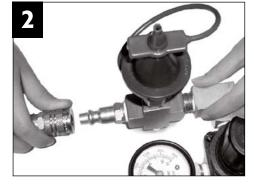
Push to connect the supply hose to the back outlet on the Dual Split-Second Sizer.
