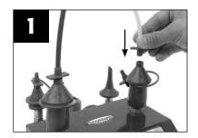
Press-fit the Double Bubble Outlet onto the inflating outlets of the Dual Split-Second Sizer. Attach the yellow hose to the right outlet and the blue hose to the left outlet.
