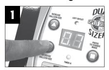
Reference the Size Setting Chart below for proper balloon sizes. Set the appropriate number of seconds by pressing the arrow buttons on the control panel digital display window.
