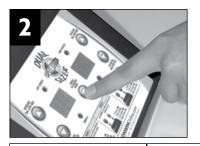
Select the proper mode by pressing the "PRESS TO CHANGE MODE" button. The LED display will indicate which mode the Dual Split-Second Sizer is in. (See MODE Chart Below)
