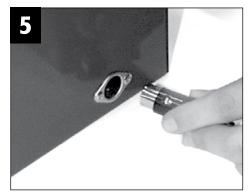
Plug the foot pedal into the side of the unit.
