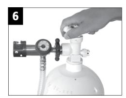
Slowly open the cylinder valve. Make sure the valve is fully opened. The cylinder pressure will read on the gauge located on the regulator. The inlet pressure will read on the second stage regulator gauge, located on the back of the unit.
